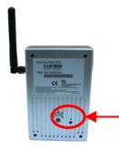
button in the back of the Network Camera. It is used to reset the system or restore the factory default settings. Sometimes resetting the system sets the system back to normal state. If the system problems remain after reset, restore the factory settings and install again.
